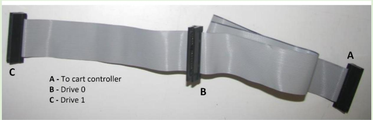
the orientation of the cable, just that the drive should be connected to the innermost connector (B) from the drive end of the cable. I assumed this was for drive 0 and the connector at the end of the cable was for drive 1. The image above shows the drive cable, labeled using the same nomenclature as used in the Tandy reference manual.
