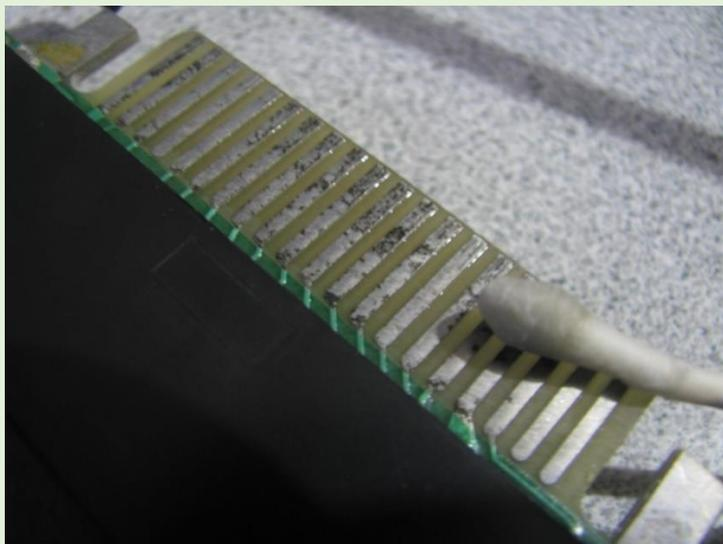
Some of the connectors were dirty. The Q-tip became soiled as I gently stroked the metal strips. Note: Q-tips aren't the best tool for cleaning. They bend easily, even with light pressure. After cleaning them I retested, making sure all the connectors were dry. This had no effect on the drive's behavior.
