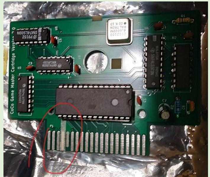
While I chose to hack on a jumper and header for pins 7 and 8, Steve chose the venerable trick of putting tape on top of pin 7 to sever the connection to pin 8, as is highlighted by the red circle in the image.
