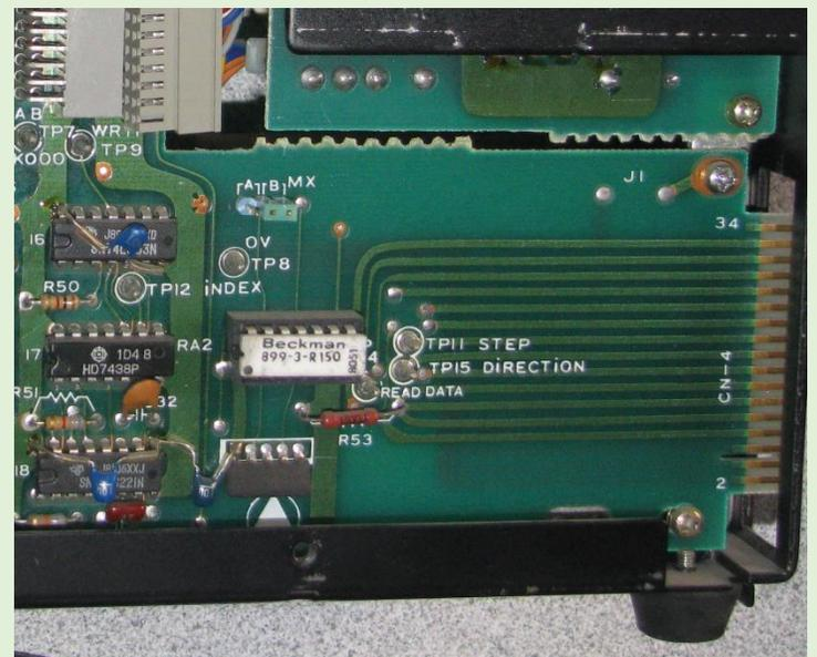
The above image clearly shows the floppy drive's edge connector and pin 2 at the bottom of the drive and close to the notch. Pin 1 located!
